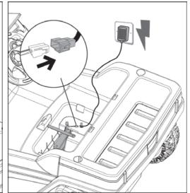
**NOTE:** It is not necessary to remove the battery for charging. However, if the battery does not reach the outlet, it can be removed for charging. For battery removal, see step 3.
