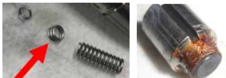
Figure 16. Broken spring (left) and corroded plunger (right).
