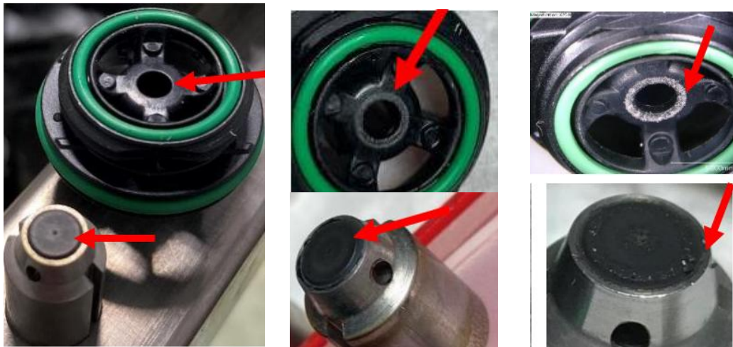
Figure 15. No wear (left), moderate wear (centre), heavy wear (right).
