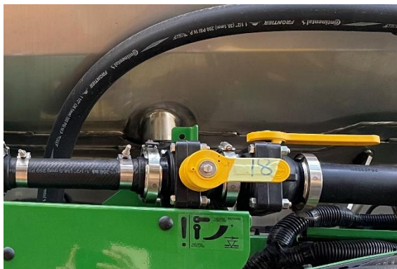
Figure 4. Orifice Valve in open position
